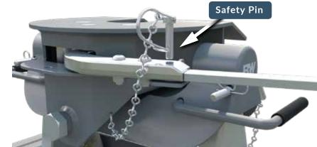
4. Use the safety pin to lock the handle in the open position and when you are sure that the landing gear will support the trailer, move the truck forward to release the jaws from the kingpin.
