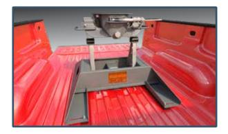
2. Swivel the locking bracket from over the drawdown bolt head. Loosen the drawdown bolt.
