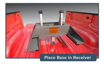
**3.** Tighten the drawdown bolt on the top of the square post to 60 ft-lbs. Lock the drawdown bolt in place by swiveling the locking bracket over the bolt head. (Flatbed models - 40ft-lbs)
