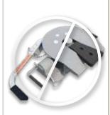
Preventing the kingpin from rotating within the jaws of the Companion coupler with a wedge, or any other device, such as Reese Sidewinder® or Reese Revolution®, could result in property damage, serious injury or death.
