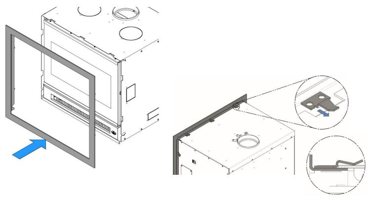
3. Make sure the fan cord is out on the side, in the opening between the front and the insert.
