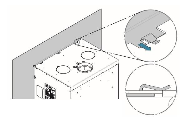
3. Make sure the fan cord is out on the side, in the opening between the front and the insert.
