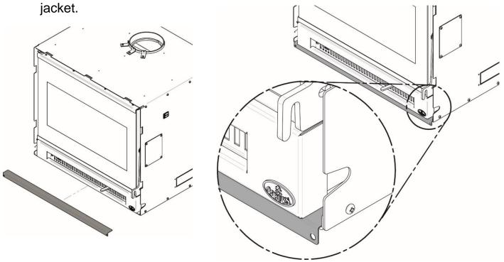
2. Align the clips on the faceplate with the notches on the insert. Push the front panel onto the insert until it snaps onto it.
