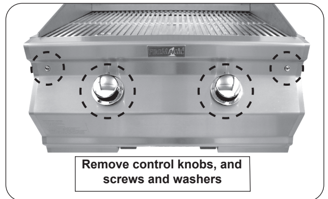
Fig. 28-3 Remove knobs and screws
