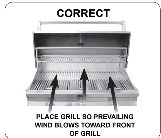
Fig. 14-2 Airflow direction - CORRECT
