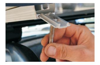
2. Slide the bolts and channel sliders into the mounting channels. You will need to lift your rooftop tent side, so as to have one of the bolts on the inside of the roof rack. Repeat the same steps for the remaining three sides.
