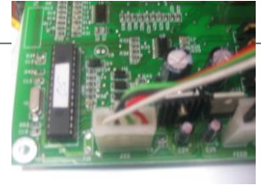
Remote Receiver Connected to Control Panel
