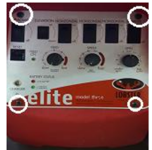
4 Control Panel Screw locations.
