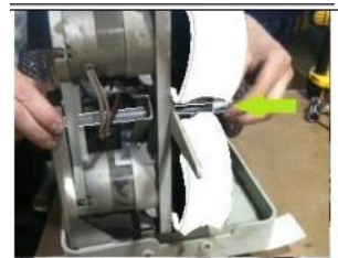
The Yoke Bolt being removed.
