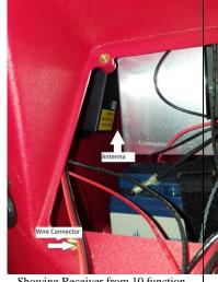
Showing Receiver from 10 function remote (physical remote assembly).
