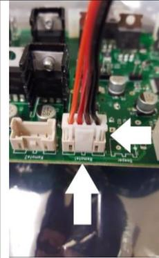
"J3" or "Remote 1" tab on circuit board. For 10 function physical remote ONLY.
