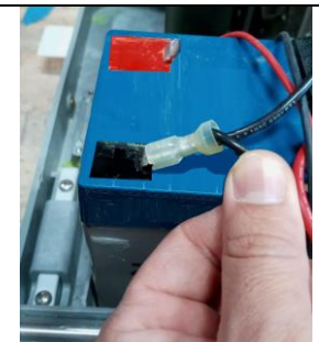
Negative wire being disconnected from Battery.
