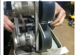
Put the Yoke on just like you took it off. Don't forget the spacers!
