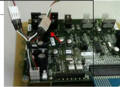
20 function remote receiver plugged into Y-Pig-Tail
