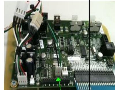
Green and white wire couple plugged into J6 connector jack, with additional Y-Pig-Tail housing both red and white Wi-Fi receiver and 20 function remote receiver.
