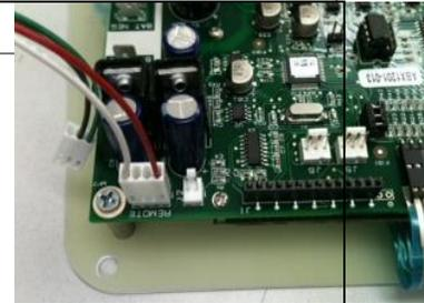
Wi-Fi red and white wire couple plugged into Remote connector jack.
