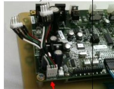
Y-Pig-Tail attached to 4-prong Remote connector jack.
