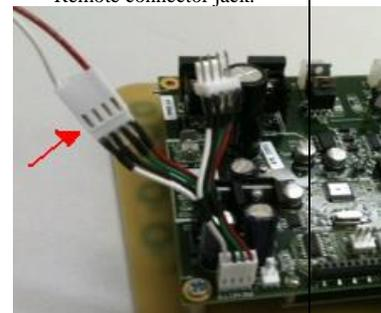
Red and white Wi-Fi female plugged into Y-Pig-Tail.
