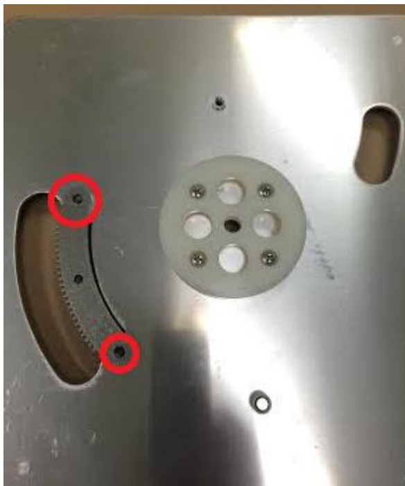
Arc Gear screw holes (marked in red)
