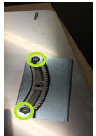
Kep Nuts holding shield to Arc Gear (marked in Green)
