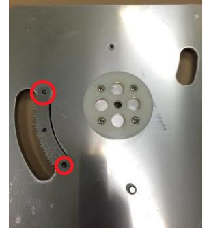
Arc Gear screw holes (marked in red)
