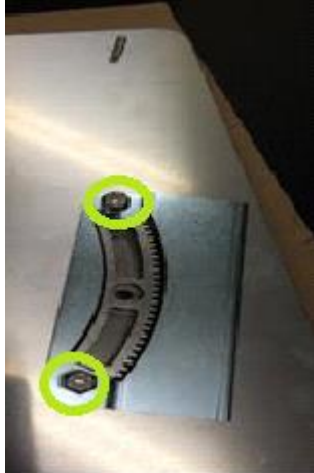
Kep Nuts holding shield to Arc Gear (marked in Green)
