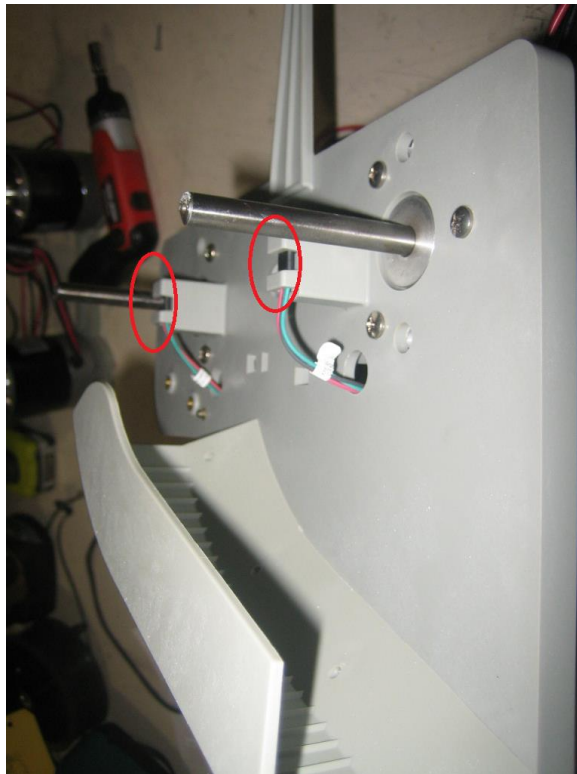
Top and Bottom Server Motor Snap-in Sensor Wires
