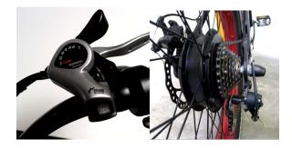
When the shifter is in the 7th position the sprocket should be on the smallest sprocket.
