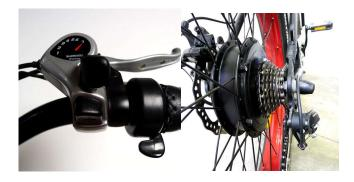
Occasionally the shifter gear number and sprocket locations may not match. If this happens then the derailleur needs an adjustment. Adjustments can and should be done by a qualified bicycle technician.
