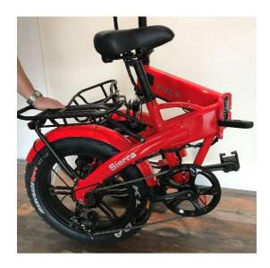
3. To fold the handlebars, pull the safety latch down and gently pull the handlebars down to the right side of the bike.
