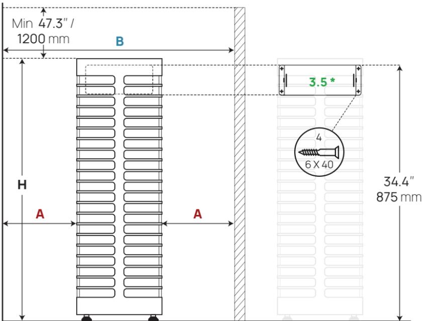
\* STEEL Mini 3.5 is attached to the wall with a special bracket
