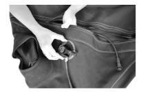
• Twist the valve into the connector and put the connection cable and connector through the hole for the valve to the inside of the suit.
