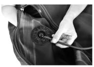
Turn the suit so the inside part is visible and put the connection cable through the nut that will hold the valve. Twist the nut onto the valve until strong resistance, to make sure it will not leak.
