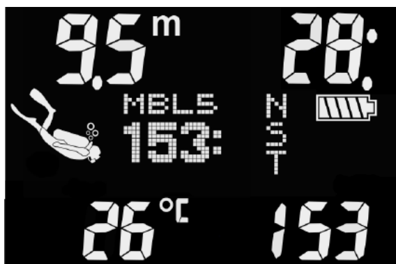
No -stop time and MB-level (ADT algorithm)
