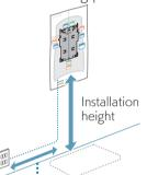
Length obtained by subtracting installation height from cord length (about 6.6 ft) of AC adapter
