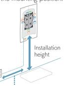
Length obtained by subtracting installation height from cord length (about 6.6 ft) of AC adapter
