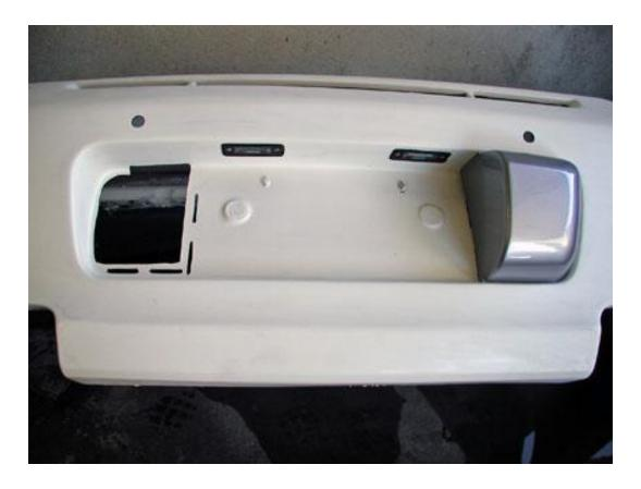
If you want to use the bumper guards, it will be necessary to modify bumper as picture shows. Slot and cut opening in license area to install bumper buffers. We recommend using a small amount of adhesive in the slotted part of the bumper.
