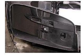
Remove original cooler/condenser shrouds and replace them with the GT shrouds provided with your kit. It may be necessary to trim the GT shrouds to install. Install and wire got lights that are attached to the back of the shroud openings.
