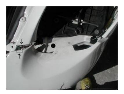
Attach GT front bumper to fender in slotted area at front of fender, fixing lock slider to hold bumper in place. Lock slider should be installed on to the fixing plate through opening in inside leg of fender, next to hood. This will hold the front fender to bumper. Now attach bumper in front of hood with factory screws.
