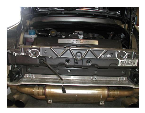
Rear panel can be raised or lowered by loosening speed nuts. Holes in panel can be enlarged to allow for more adjustment. Bumper will be raised or lowered by moving the panel up or down.
