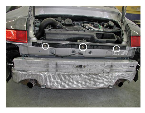
Rear panel above reinforcement can be adjusted up or down when fitting GT Rear Bumper. Ends of reinforcement need to be trimmed to clear Turbo intercooler covers. Exhaust muffler outlet pipes need to be moved so they line up in center of exhaust outlets in the diffuser.
