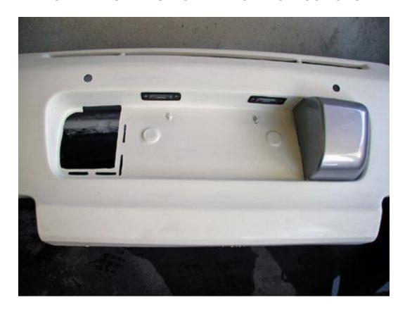
It will be necessary to slot and cut opening in license area to install bumper buffers. We recommend using a small amount of adhesive in the slotted part of the bumper.
