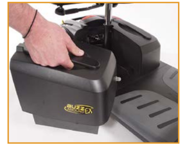
Step 2: Pull out the battery pack!
