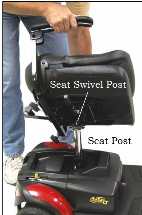
Figure 23. Installing the Seat
