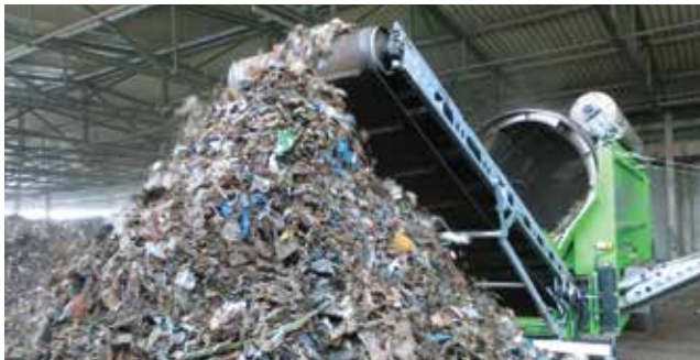
Star screen insert. 1 piece fines belt prevent spillage at transfer point
