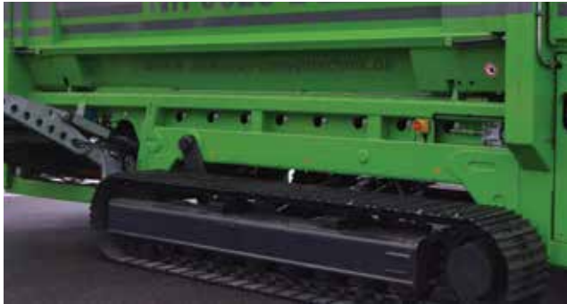
Track Risers • Raise or lower the machine • Tilt front to back
