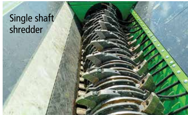
Adjustable gap between shaft & counter comb for continued shredding action
