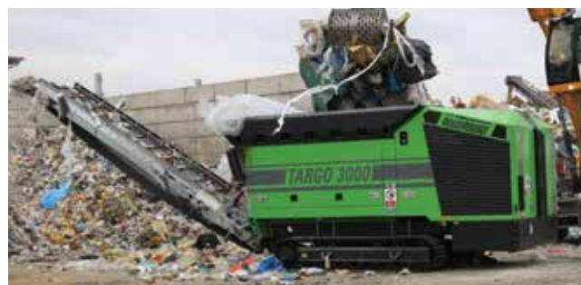
Adjustable gap between shaft & counter comb for continued shredding action
