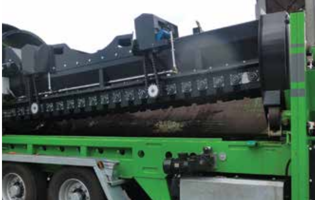
Star screen insert. 1 piece fines belt prevent spillage at transfer point
