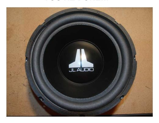
\*\*Allow 24-36 hours for adhesive to fully cure before placing a full load on your newly-refoamed speaker.
