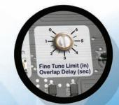
Innovative fine tune adjustment for the end of gate travel ( down to 1/8")
