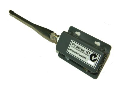
The R-2000 Ultra Long Range RFID Reader detects and decodes RF transmitted signals from 1st Choice Tags.
