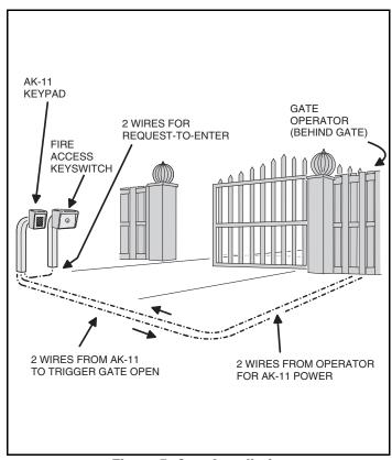
Figure 5. Gate Installation
