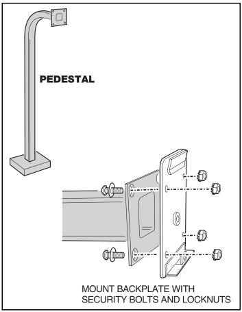
Figure 3. Pedestal Mounting Keypad Backplate
