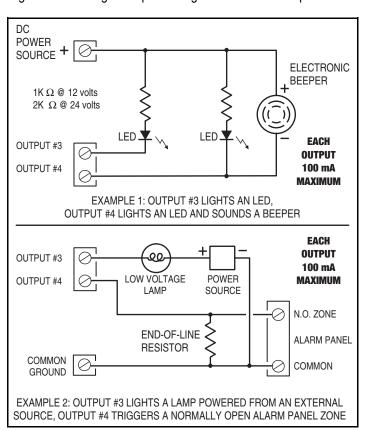
Figure 7. Using the Solid State Outputs
