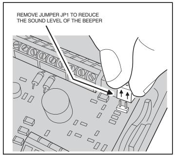
Figure 8. Removing Beeper Jumper
