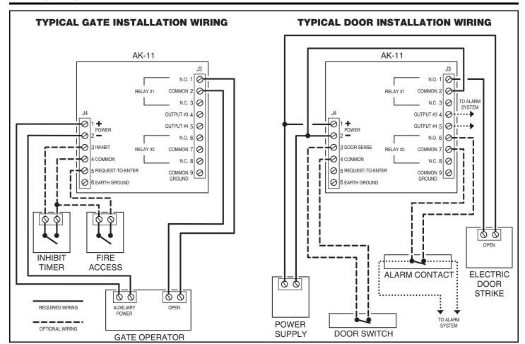
Figure 2. Wiring Diagram
