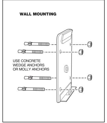
Figure 4. Wall Mounting Keypad Backplate
