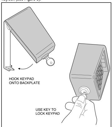
Figure 9. Locking the Keypad Case
