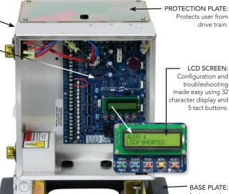
LCD SCREEN: Configuration and troubleshooting made easy using 32 character display and
