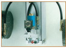
Bypass solenoid unit. Allows the beam to be opened manually in the event of a power failure.
