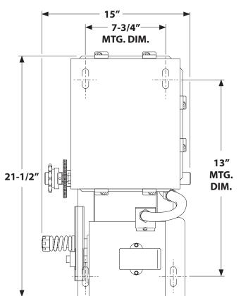
HEAVY DUTY V-BELT AND CHAIN REDUCTION, MECHANICALLY SELF LOCKING
