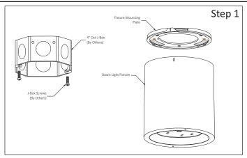
**Step 1** - Disassemble Luminaire Parts for easy Installation: a.- Remove Mounting Plate from Down Light Fixture by turning
