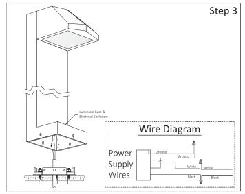
Step 3 - Make Wiring Connections:
