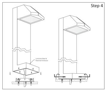
Step 4 - Install Luminaire LED Enclosure to Base:
