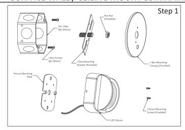
**Step 1** - Disassemble Luminaire Parts for easy Installation:
