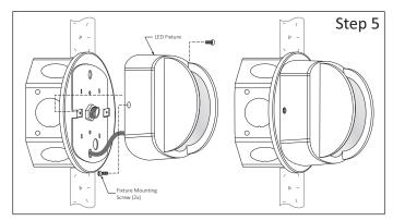
Step 5 - Install LED Fixture:
