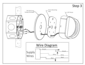
Step 3 - Make Wiring Connections:
