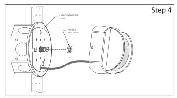
**Step 4** - Install Fixture Mounting Plate:
