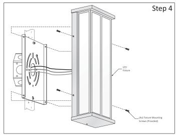
Step 4 - Install LED Fixture:
