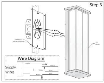
Step 3 - Make Wiring Connections:
