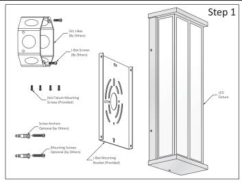
**Step 1** - Disassemble Luminaire Parts for easy Installation:
