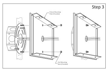
**Step 3 -** Install Fixture Mounting Plate: a.- Run Input wires through center hole of Mounting Plate. b.- Insert the two 8-32 Screws (provided) through the Holes and use the Nuts (provided) to secure the Plate on Mounting Surface. READ AND UNDERSTAND ALL INSTRUCTIONS BEFORE INSTALLATION. IF YOU ARE NOT FAMILIAR WITH THE NATIONAL ELECTRICAL CODE (NEC), CONTACT A QUALIFIED ELECTRICIAN TO INSTALL THIS LUMINAIRE.
