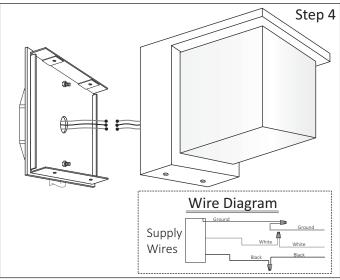
Step 4 - Make Wiring Connections:
