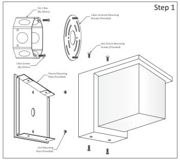
**Step 1** - Disassemble Luminaire Parts for easy Installation: a.- Remove Fixture Mounting Plate and Bracket from Fixture.
