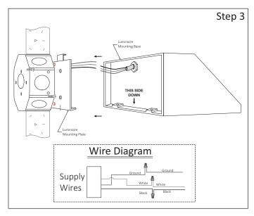
**Step 3** - Make Wiring Connections:
