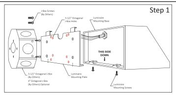
**Step 1** - Disassemble Luminaire Parts for easy Installation:
