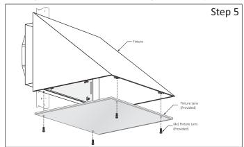
Step 5 - Install Fixture Lens:
