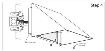
Step 4 - Install LED Fixture:
