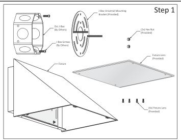
**Step 1** - Disassemble Luminaire Parts for easy Installation: a.- Remove and disconnect LED Fixture from Mounting Base.
