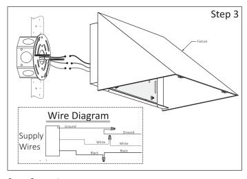
**Step 3** - Make Wiring Connections:
