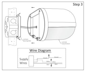
Step 3 - Make Wiring Connections:
