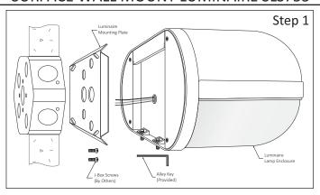
**Step 1 -** Disassemble Luminaire Parts for easy Installation:
