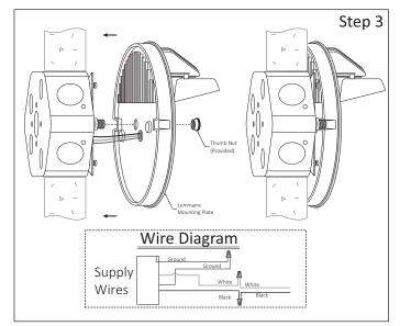
**Step 3 -** Make Wiring Connections/Install Mounting Plates: a.- Run the Electrical Wires through all the Parts and make hard-wire connections, see Wire Diagram.
