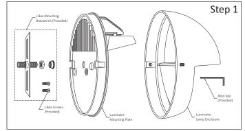
**Step 1** - Disassemble Luminaire Parts for easy Installation: a.- Remove Mounting Plate to install Luminaire Lamp Enclosure.
