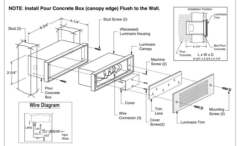
RECESSED LUMINAIRE - WALL MOUNT SL 300 STEP LIGHT Series -
