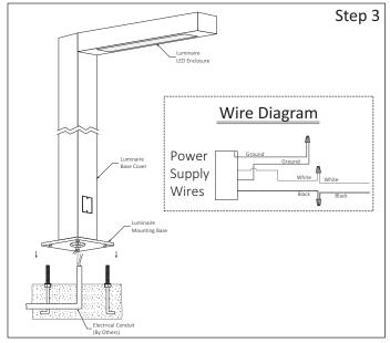
Step 3 - Make Wiring Connections: a.- Place Luminaire Base close to the Mounting Surface and make hard-wire connections, see Wire Diagram.
