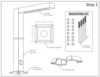
**Step 1** - Disassemble Luminaire Parts for easy Installation: a.- Get Familiar with all Mounting Parts before setting the Installation.
