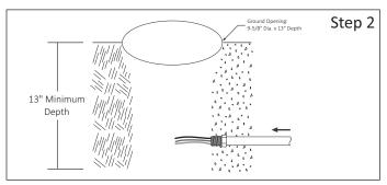
**Step 2 - Prepare In-Ground Opening for CPX Box:**
