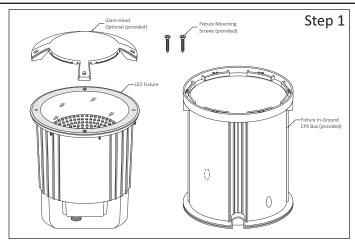
**Step 1** - Remove Luminaire Parts for easy Installation: a.- Remove the LED Fixture from CPX Box and two Mounting Screws. **NOTE: Do Not open the LED Fixture for Installation!!!**
