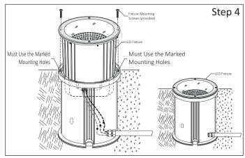
Step 4 - Install LED Fixture:
