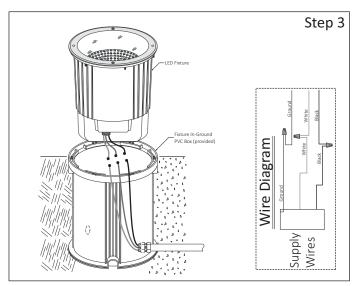
Step 3 - Install In-Ground Box & Make Wiring Connections:
