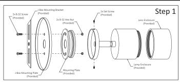
**Step 1** - Disassemble Luminaire Parts for easy Installation: a.- Remove Mounting Plates and Lens Enclosure if need to install Lamp.
