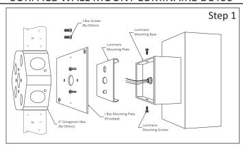
$\begin{tabular}{ll} Step 1 - Disassemble Luminaire Parts for easy Installation: \\ \end{tabular}$
