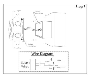
Step 3 - Make Wiring Connections:
