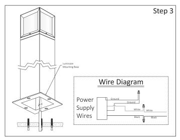
Step 3 - Make Wiring Connections:
