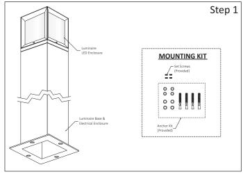
**Step 1** - Unpack all Luminaire Parts for easy Installation: a.- Check Luminaire Mounting Base and Anchor Kit (Provided).
