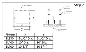
Step 2 - Install Luminaire Mounting Anchor Kit:
