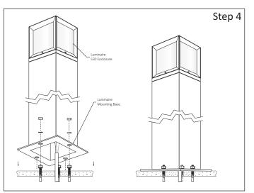
Step 4 - Install Luminaire Base:
