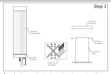
**Step 1** - Disassemble Luminaire Parts for easy Installation: a.- Remove Luminaire Base and Lens Enclosure to install Lamp.
