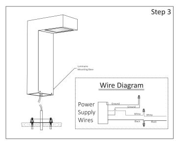
**Step 3 - Make Wiring Connections:**
