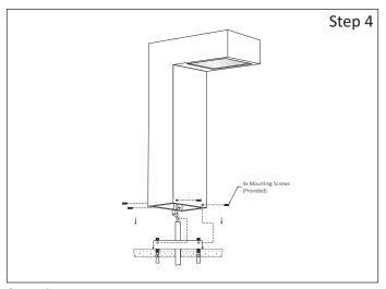
**Step 4** - Install Luminaire Mounting Base:
