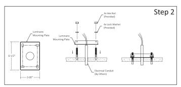
Step 2 - Install Luminaire Mounting Plate:
