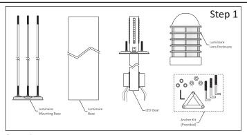
**Step 1** - Disassemble Luminaire Parts for easy Installation: a.- Remove Luminaire Base and Lens Enclosure to install the Base.
