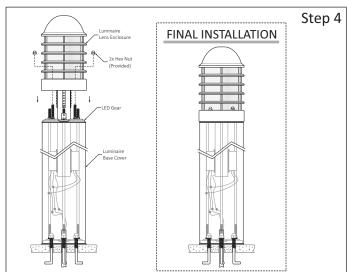
**Step 4** - Install Luminaire Lens Enclosure:
