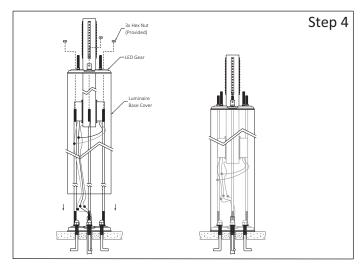
**Step 4** - Install Luminaire Base Cover:
